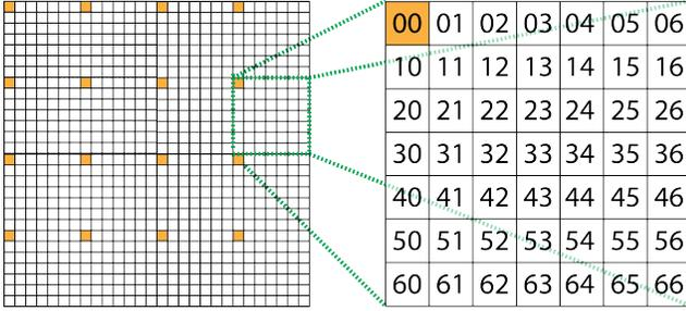
**Figure 2: An example matrix layout for CAPS.** Each of the 16 submatrices as shown on the left has exactly the same layout. The colored blocks are the ones owned by processor 00. On the right is a zoomed-in view of one submatrix, showing which processor, numbered base 7, owns each block. This is block-cyclic layout with some blocksize  $b$ , and matches our layout requirements with parameters  $(n = 4 \cdot 49 \cdot b, P = 49, s = 2)$ .
