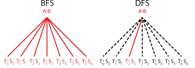
**Figure 1: Representation of BFS and DFS steps.** In a BFS step, all seven subproblems are computed at once, each on  $1/7$  of the processors. In a DFS step, the seven subproblems are computed in sequence, each using all the processors. The notation follows that of Appendix A.
